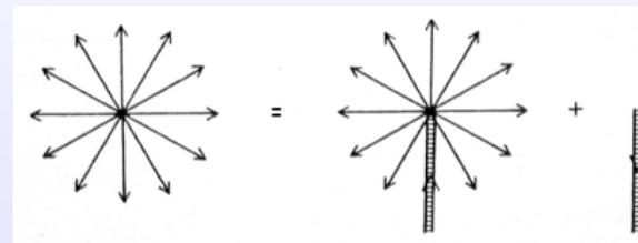
Add an infinitely small, infinitely extended solenoid field (e.g. along the negative z-axis):
